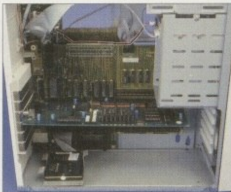
Now it's simply a matter of connecting the various plugs and leads to your drives and the motherboard and busboard and you're nearly there. Notice the already installed 24-bit Zorro expansion card. Try fitting that into a standard A1200, matey!
